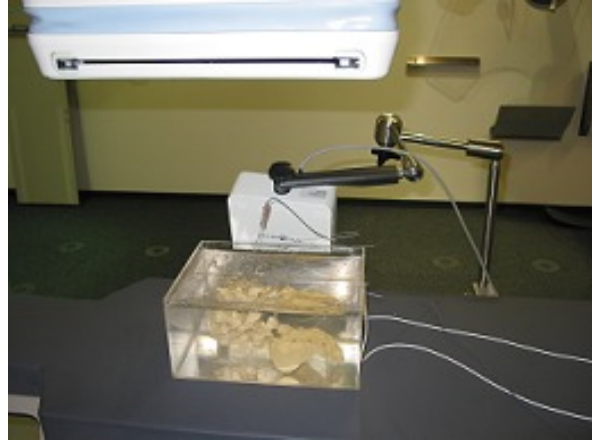
Fig. 2b. Wax phantom with simulated lesions
