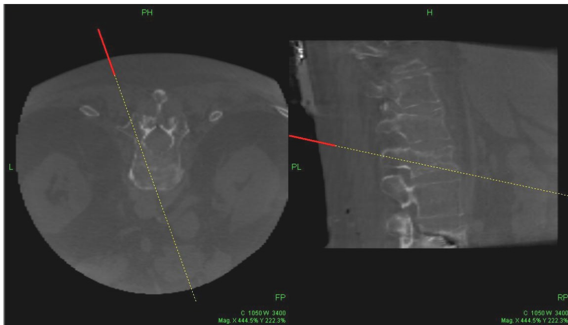
Fig. 6. Screenshot during introducing the kyphoplasty needle. The dotted line marks the extrapolation of the needle in forward direction. The left and the right part of the image show a transversal and a sagittal view of the spine, respectively. The needle target is the collapsed vertebra to be reconstructed.
