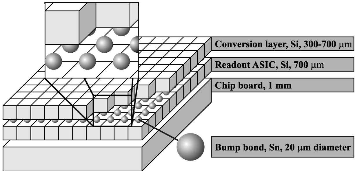
**Figure 2.** Principal setup of the simulated detector. The semiconductor conversion layer is bump-bonded to the readout chip by flip-chip technology. The chip board is also implemented.
