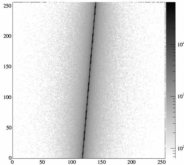
**Figure 4.** A typical simulated LSF image of a Medipix2 assembly. The LSF image was simulated using  $10^9$  photons with an energy of 30 keV.
