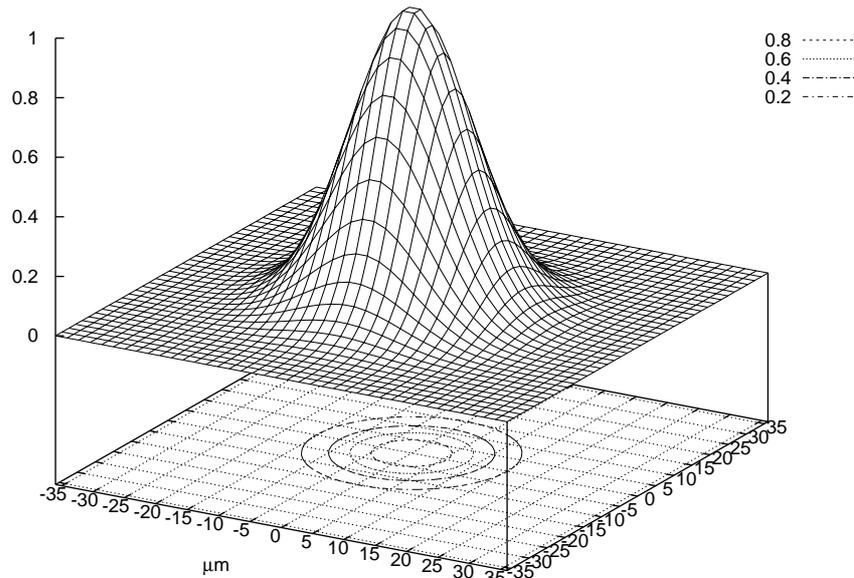
**Figure 3.** This figure shows one possible PDF for modeling the charge carrier transport inside the semiconductor. The charge is distributed over an area of several  $\mu\text{m}^2$ .
