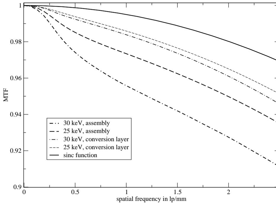
**Figure 6.** Calculated MTFs as a functions of spatial frequency. All simulations were carried out with  $10^9$  photons. From the simulation of the assembly a LFD can be observed. The sinc function as a upper limit for the MTF is plotted for comparison.
