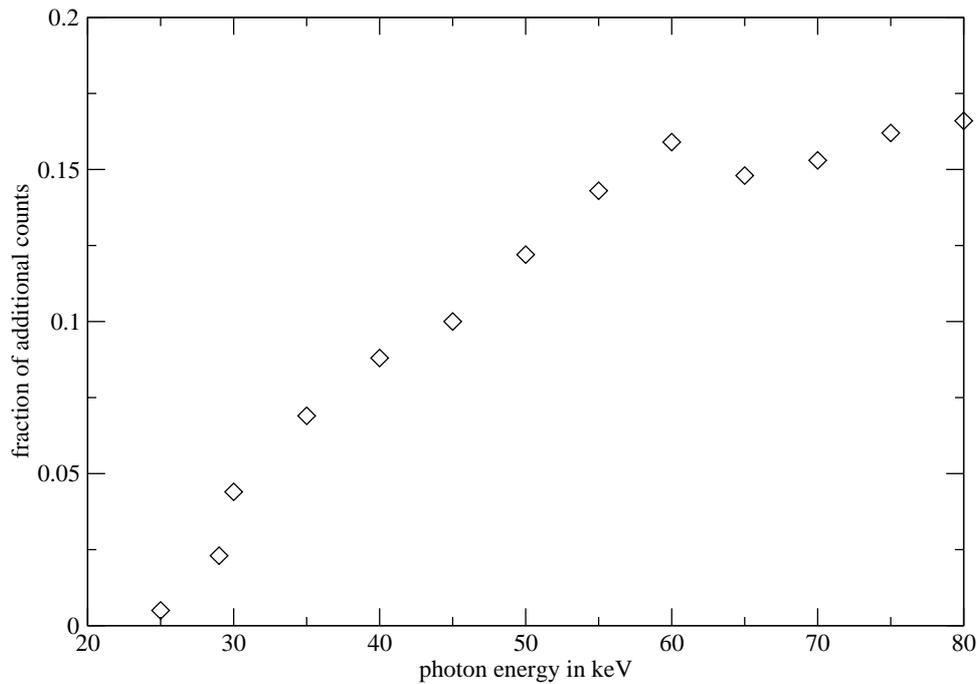
**Figure 5.** Fraction of additional detected events as a function of the incident photon energy. For higher energies more photons are transmitted through the conversion layer. Therefore, more photons hit the bump bonds and more fluorescence photons are generated.
