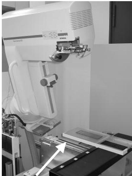
Figure 2: Mammography system with linear array detector (arrow) and sample carriage.
