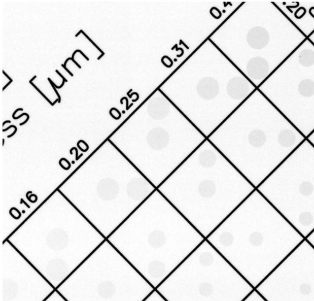
Figure 7a: Details of the CD-MAM phantom imaged with polychromatic radiation.
