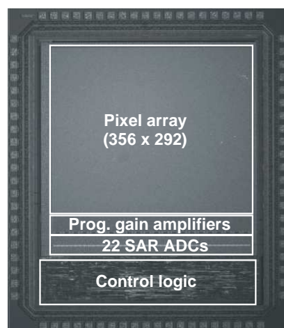
Figure 8. Micrograph of a digital single-chip camera with a power consumption of less than
