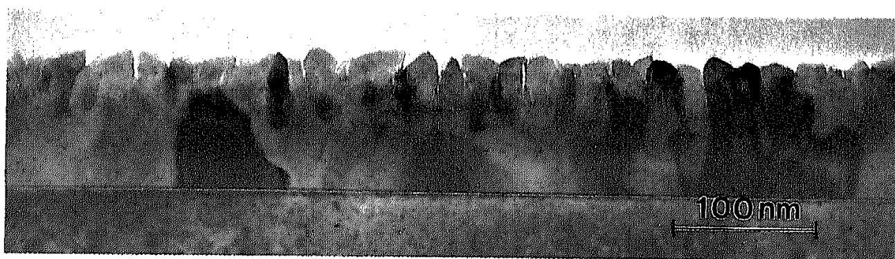
Fig. 4. The restricted reproducibility of ITO film fabrication ( p[\text{O}_2] = 1.6 \times 10^{-1} Pa) is demonstrated by the different microstructure compared to Fig. 2
