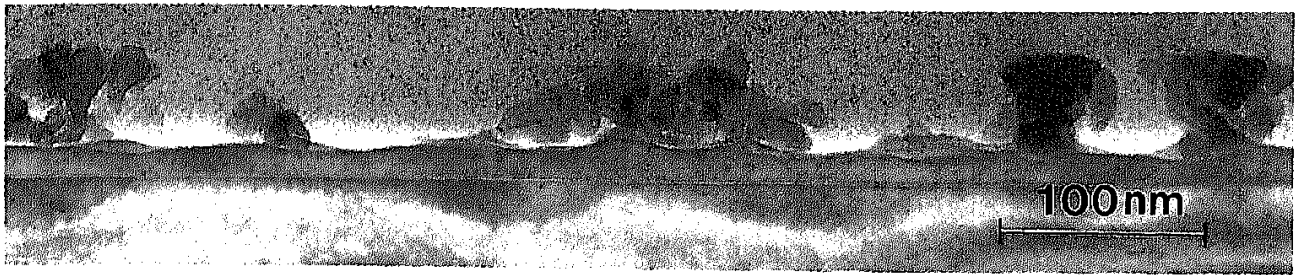
Fig. 7. Polycrystalline ITO film after prolonged exposure to etching agent
